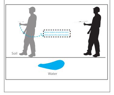
There is another way to locate the water location more accurately, (Square method) take 4 different readings for the target from 4 angles forming a square 3 m from water location the intersection point of the for readings is the water location.
